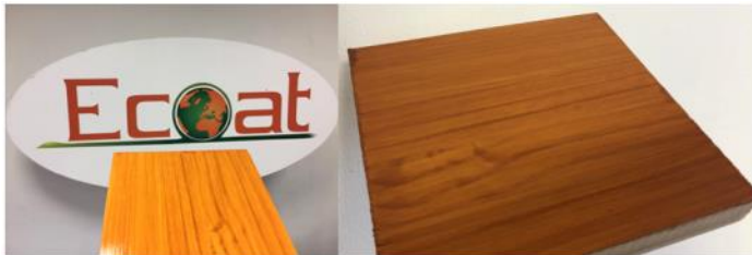
Figure 2: Pine wood panel coated with Inokem UR 3304 as a top coat.
