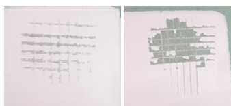
Figure 4: Cross cut test adhesion on plasterboard of Secoia 1400 and a styrene acrylic.
