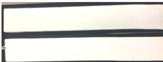
Figure 3: Mate paints after wet scrub resistance test.
