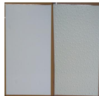
Figure 4: Paint after 240h in QCT test (ISO 6270) - Left side: Inokem UR 3301 - Right side: Solvent-based urethane alkyd paint.
